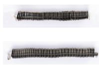
Weight per Unit of Length for Chips Generated by the Inner Edge (In-house Evaluation)
